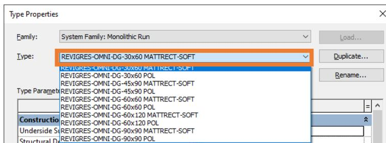
After choosing the type of object of the **DG** typology, it is necessary to change the material for the step itself will be chosen in the **Materials and Finishes** section in the parameter **Tread Material**:
