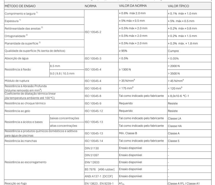
permissible deviation of the average value for each tile from the work size (w); 2) deviation related to corresponding work sizes;
